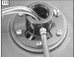
Loosen 2 screws and remove pin with keeper for downrod, yoke cover, and canopy to fit in yoke of fan.
